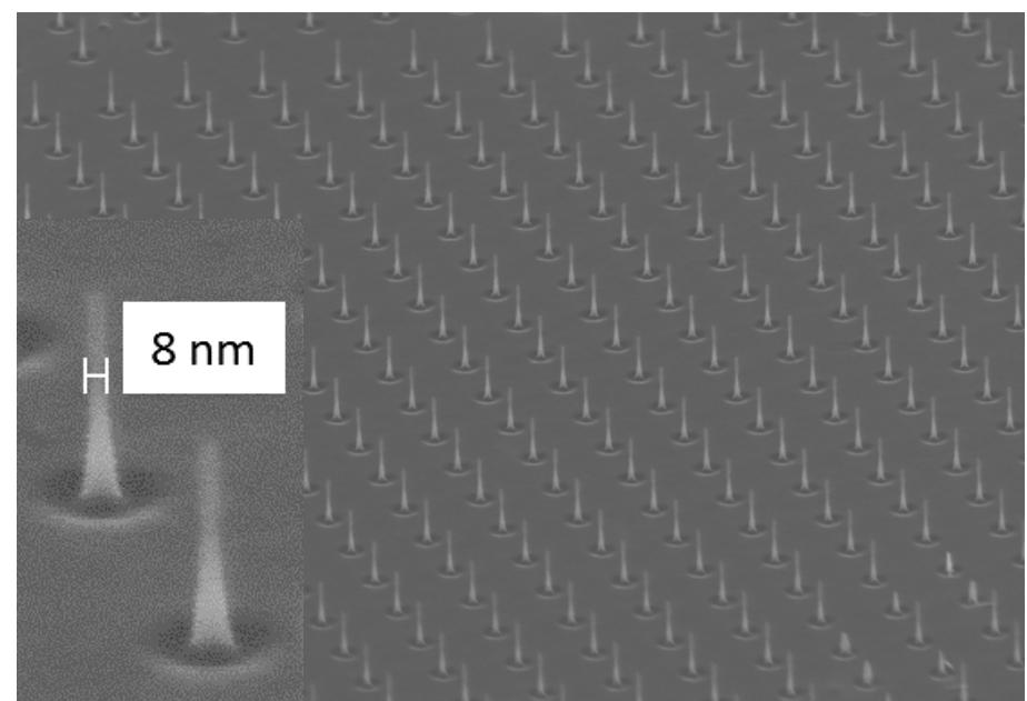
Alcohol-based DE enables  $D < 10$  nm
