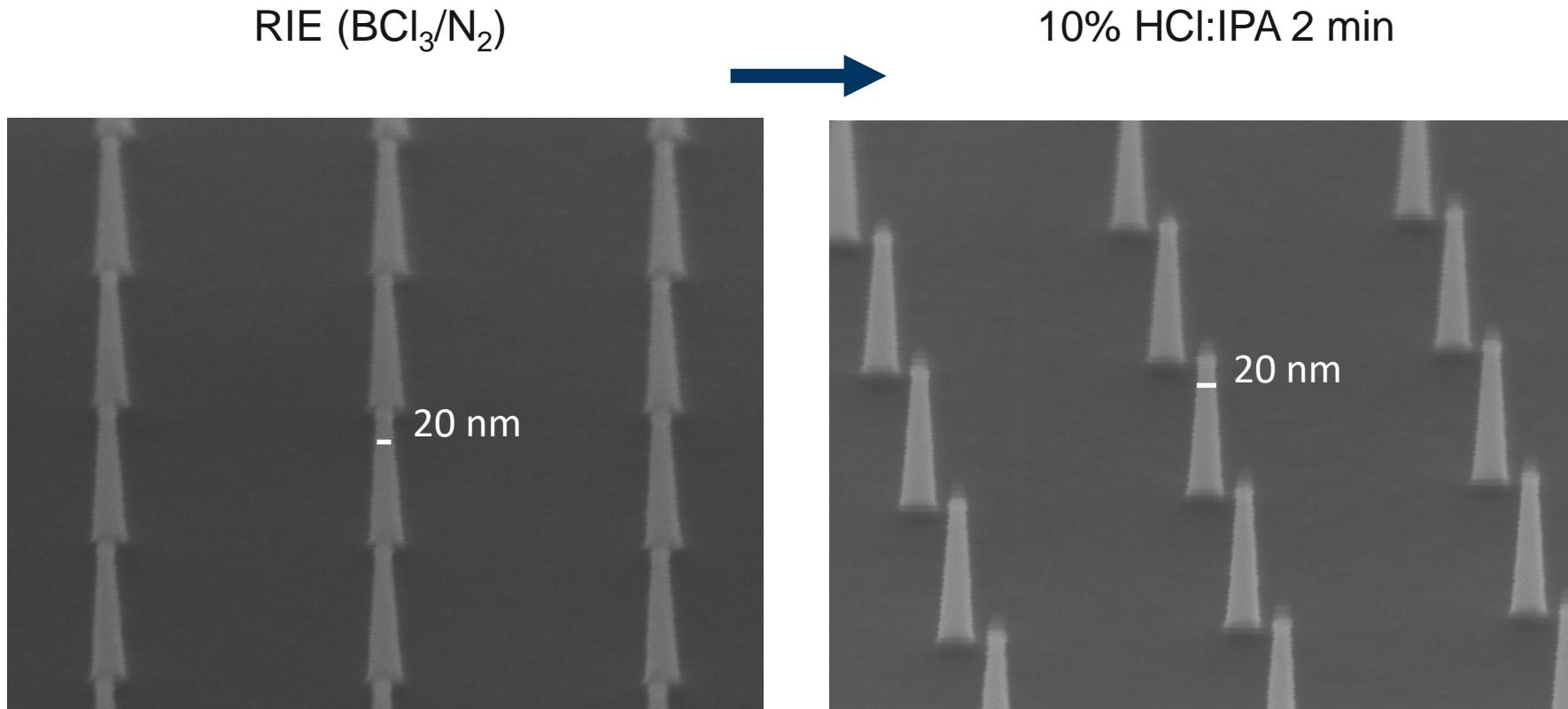
Alcohol-based HCl treatment does not damage III-Sb sidewall
