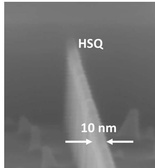
First demonstration of InGaSb DE with radial etch rate = 1.0 nm/cycle
